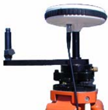
Allowing for kinematic initialization using Initializer bar at the base
